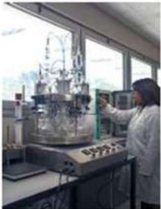
M.O.D.A.-4 for aerobic biodegradation (ISO 14855-2)
