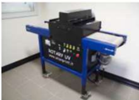
UV drying unit for surface treatment ROTARY
